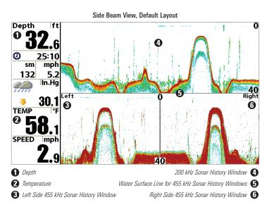
**Classic layout:** The top portion of the display presents a historical log of sonar returns from the 200 kHz down-looking sonar beam. New information in the down beam panel scrolls from right to left. The bottom portion of the display presents a historical log of sonar returns from the 455 kHz right- and left-looking sonar beams. New information appears at the top, and scrolls down the display.
