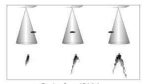
Transducer Cone and Fish Arches
