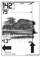
When all the echoes are viewed side by side, an easy to interpret "graph" of the bottom, fish and structure appears.
