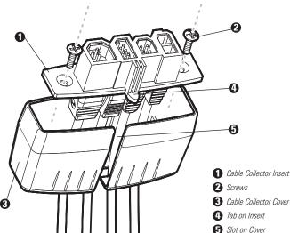
Plug Cable Connector Assembly to Back of Control Head
