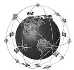
GPS uses a constellation of 24 satellites that continually send radio signals to the earth. Your present position is determined by receiving signals from up to 16 satellites and measuring the distance from the satellites.
