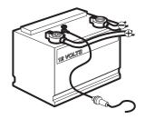
**NOTE:** Make sure that the power cable is disconnected from the control head at the beginning of this procedure.
