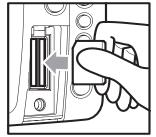
Inserting an MMC/SD into the Card Slot
