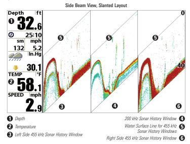
In all of these layouts, the sonar information from the side-looking beams reveals bottom contour, structure and fish similar to the down-looking beam, but the area covered is to the left and right of the area shown in the down-looking portion, so you actually see more of the bottom. The distance covered by the right and left beams is based on the depth setting for the down-looking beam, up to a maximum of 160 feet.
