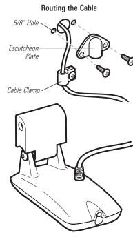
3. Place the escutcheon plate over the cable hole and use it as a guide to mark the two escutcheon plate mounting holes. Remove the plate, drill two 9/64" (3.5 mm) holes, then fill both holes with marine-grade silicone sealant. Place the escutcheon plate over the cable hole and attach with two #8 x 5/8" (16 mm) wood screws.
