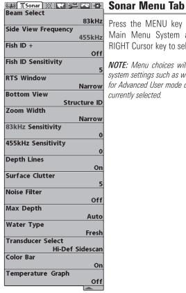
Press the MENU key twice to access the Main Menu System and then press the RIGHT Cursor key to select the Sonar tab.
