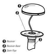
2. Screw on the receiver base to the stem first, making sure that the stem pipe does not protrude from the receiver base. This adds protection to the cable when pulling it through the pipe stem. In addition to this, de-burr the pipe edges to reduce cable abrasion.
