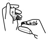
Inserting the Pivot Bolt
