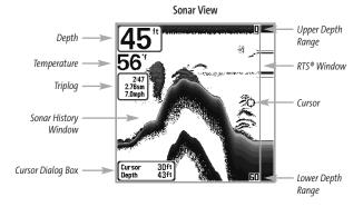
**NOTE:** If the Depth number is flashing, it means that the unit is having trouble locating the bottom. This usually happens if the water is too deep, the transducer is out of the water, the boat is moving too fast, or for any other reason that the unit can't accurately receive continuous data.
